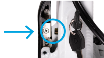
Locking Pin protruding through frame
