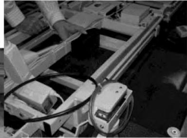
6. Locate the 4 load cell cables and plug them into the load cell jacks on the control box (see the section Specifications Control Module on page 7 for jack locations).
