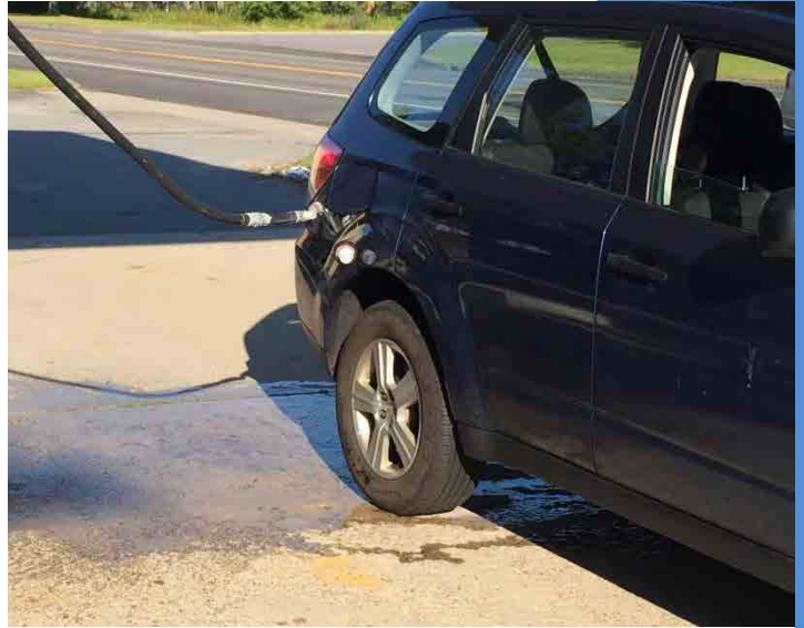
Figure 14.4: Surface spills should be cleaned up immediately. Petroleum can travel a long way in a short time.
