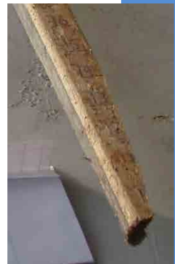
Figure 8.3: Tank gauging stick with broken end (EPA)
