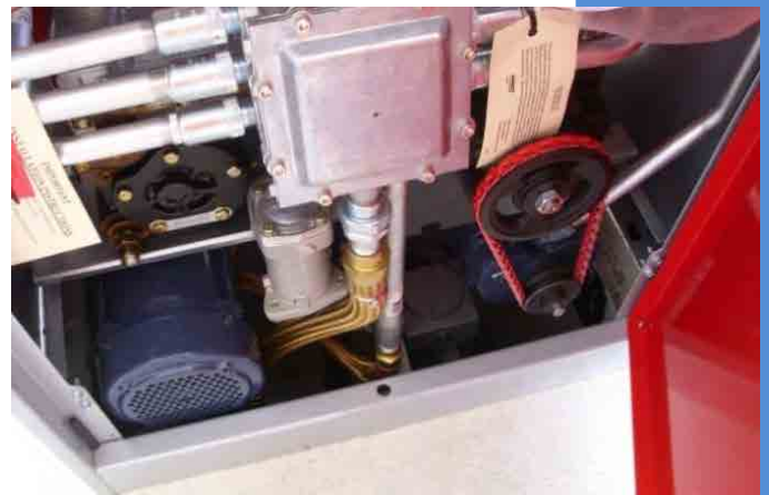
Figure 10.14: Suction system dispenser
