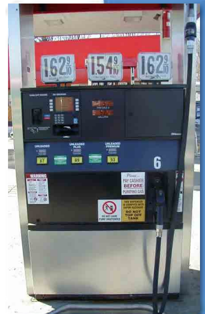
Figure 12.7: Typical retail dispenser with blending to dispense 3 grades of fuel
