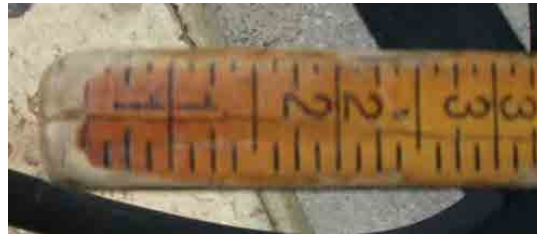
Figure 8.4: Rounded tank gauging stick (EPA)
