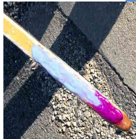
Figure 8.7: Tank gauging stick with water-finding paste. This brand turns red to indicated water level in the tank. Other brands of paste may use different colors.
